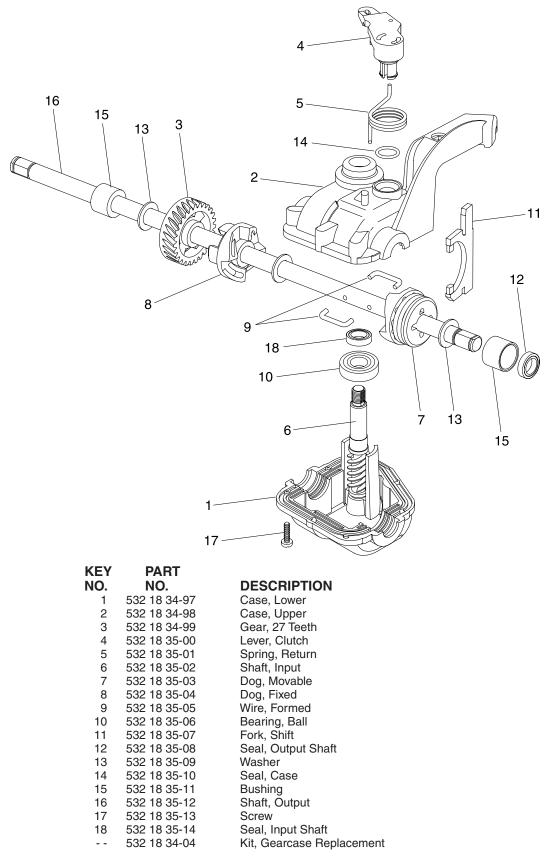
**NOTE:** Use Dow Corning #709 to reseal Gear Case Halves.
